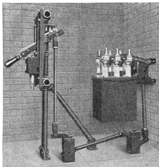
FIG. 8.—TYPE F-11, INDOOR, WALL-MOUNTING, MANUALLY-OPERATED, THREE-POLE, SINGLE-HANDLE, SINGLE-THROW, 200-AMPERE, 4500-VOLT, REMOTE CONTROL BREAKER, WITH ONE SUPPORTING LEG AND BRACE OF COVERPLATE-SUPPORTING FRAMEWORK REMOVED SO AS TO SHOW DETAILS OF CONSTRUCTION
